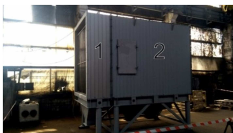
Figure 7. Combined arrangement of gas cleaning unit "MV-2-30".
