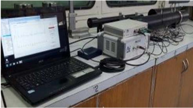
Figure 10. Impedance tube test setup.
