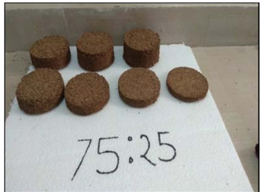
Figure 8. Test Specimen with MBWR 75.25.
