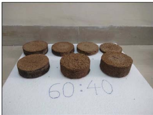
Figure 5. Test Specimen with MBWR 60.40.
