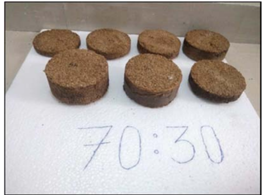
Figure 7. Test Specimen with MBWR 70.30.
