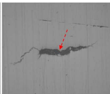
(2) Stress crack morphology
