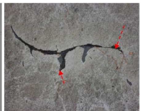
(3) The non-metallic inclusion in crack
