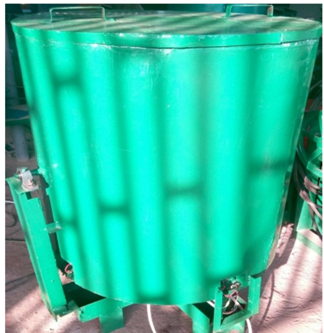
Figure 1. Pictorial view of the paddy rice parboiler.
